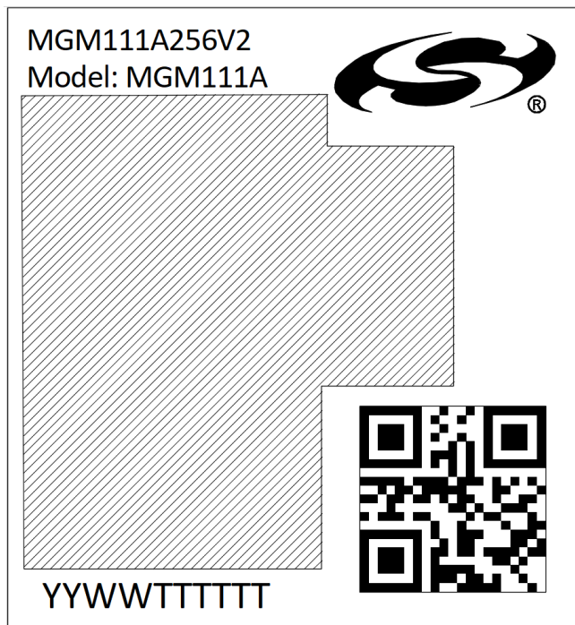
Figure 9.5. MGM111A Package Marking
